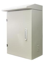
Wall-Mount Outdoor Cabinet made of sheet EG Steel or stainless steel or Aluminium make to order one by one. They can accommodate the fiber optic solution, CCTV, Broadband Cable entry 3 port use cable glands EG/PG29 depand on cable dia. The cable can be held the preformed holes, inside a 2 section cable inlet or cable feed through gromment. It can be customized to install four 4-inch ventilation fan.
