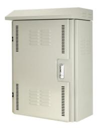
Wall-Mount Outdoor Cabinet made of sheet EG Steel or stainless steel or Aluminium make to order one by one. They can compliant with IP55-rating standard. they can accommodate the fiber optic solution, CCTV, Broadband Cable entry 3 port use cable glands EG/PG29 depand on cable dia. The cable can be held the preformed holes, inside a 2 section cable inlet or cable feed through gromment.
